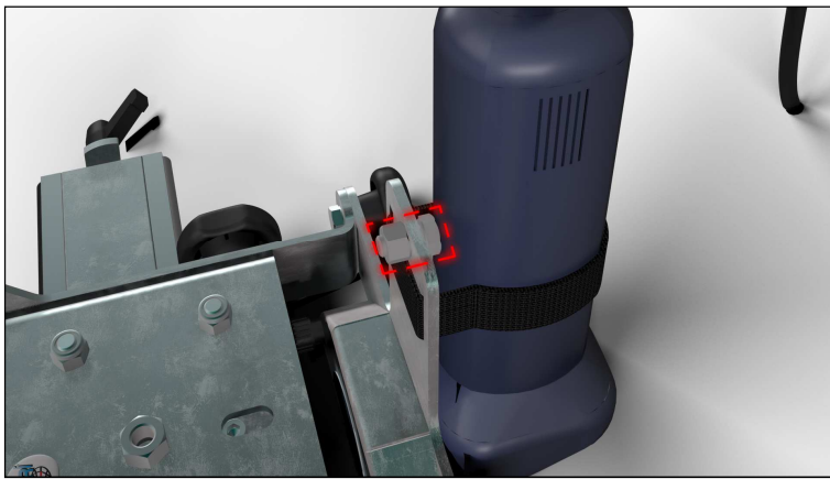
Fig. 6.4.4 Knob to adjust the crosswise movement of the carriage.
