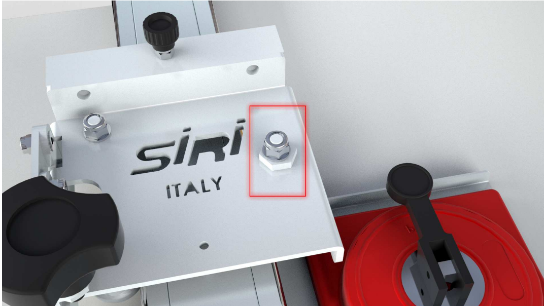
Fig. 6.4.1 Adjusting screw between guide and Siricut.
